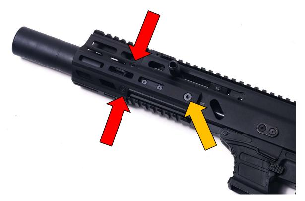
Fastening the rail continued: Tighten the rear most M-Lok mounting screws. Be sure the M-Lok T-Nuts have rotated correctly and are secured behind the M-Lok slots inside the receiver. Tighten to 30in/lb. Be sure you cannot pull up on the rail's ears to avoid snagging.
