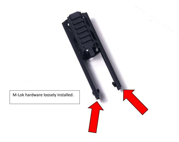
7. <u>Installing the Rail</u>: --- *This is the most difficult part of the install!* --- *Be sure the M-Lok hardware is loose!* --- Install the rail by sliding it down the sides of the receiver until in position. Be sure the rail is completely flush and seated onto the receiver. The rail should be aligned with the front sight notch, the Bridge, and rear M-Lok slots of the firearm.
